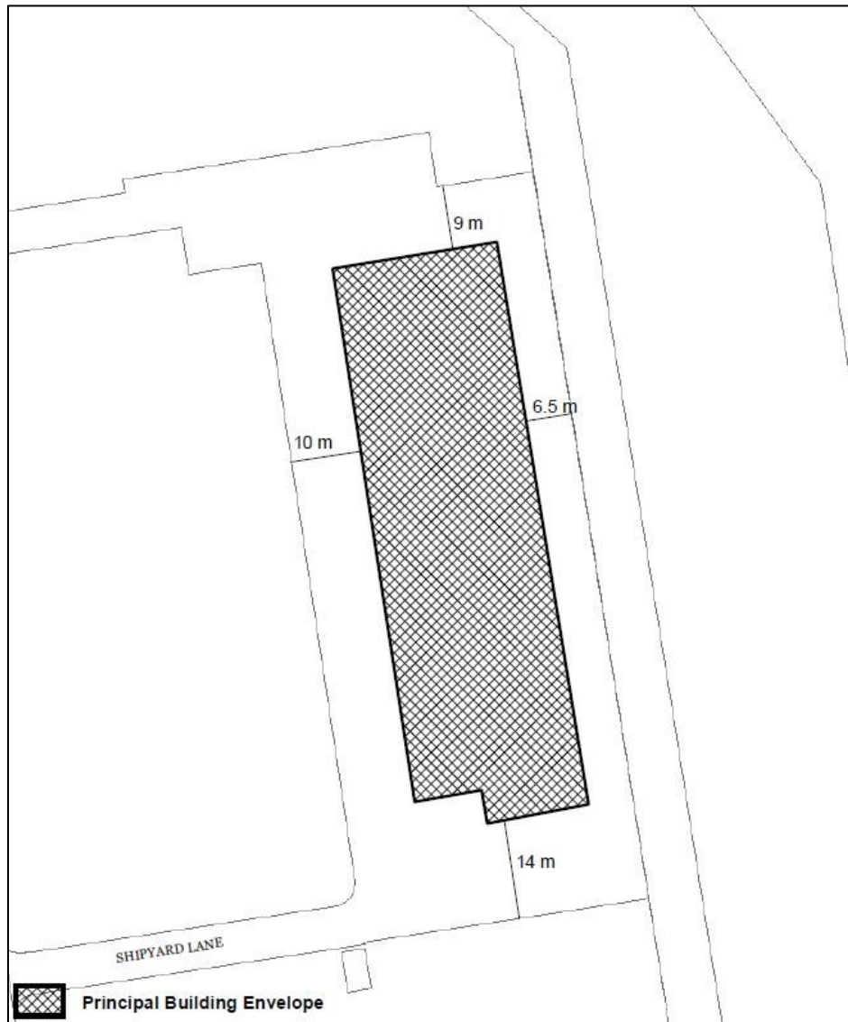
Illustration 8: R3-25 Zone requirements for building envelopes
